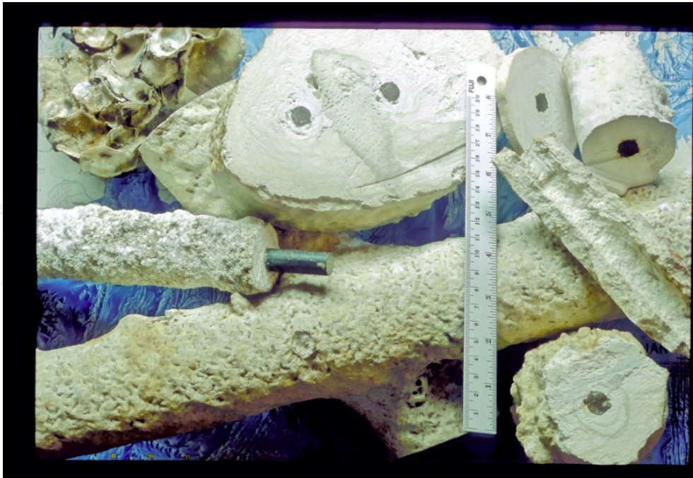
Figure 2. Biorock materials from various locations. The piece at mid left is the one shown in the previous photo. The one at top left, completely overgrown with oysters, is from Louisiana, and all the rest were grown in a two and a half year period at Ihuru Island, North Male Atoll, Maldives. Samples tested from that set of samples in the Materials Testing Laboratory of the University of Graz, Austria, had compressive strength of 60-80 Mega Pascals, around three times the load bearing strength of ordinary Portland Cement concrete. Photograph Wolf W. Hilbertz.
