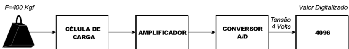
Figure 8. Relationship of physical quantity to a digital signal [3].
