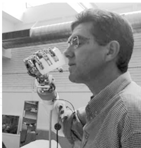
Figure 9. One of the MANUS users performing a combined cylindrical grasp and wrist rotation (extracted from [36]).
