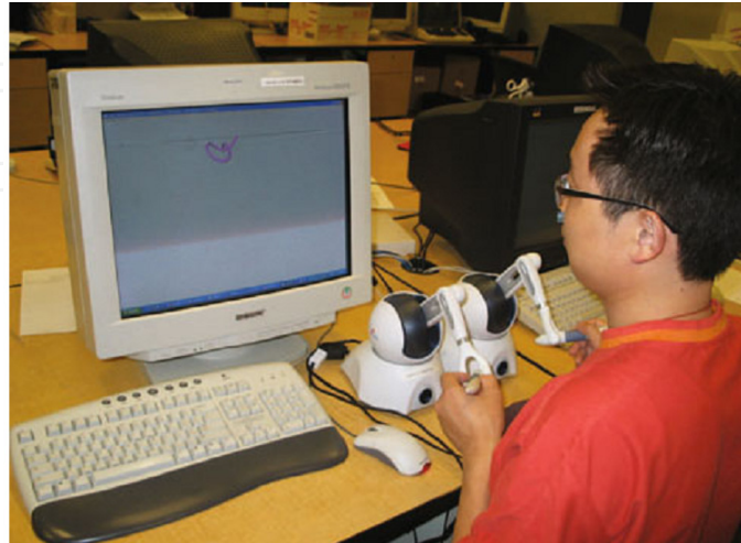
Figure 6. VR multi-modal experimental setup for simulating surgical sutures (extracted from [33]).
