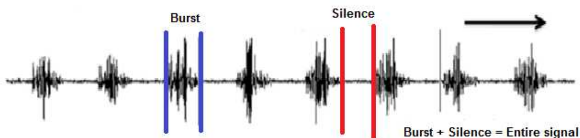
Figure 4. Burst and silence moments in an electromyography signal during a Wingate test in a cicloergometer. The break between the blue lines show a burst moment and the break between the red lines is the silence moment. Unification of Burst and Silence generates the full signal.
