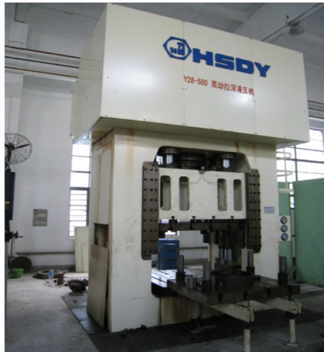
Figure 18. Dual-action deep drawing hydraulic press
