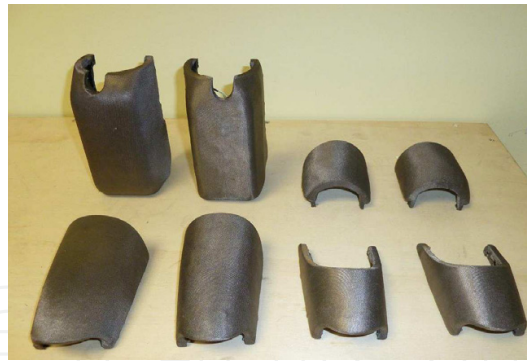
Figure 14. The covers of iCub arms covered with conductive lycra
