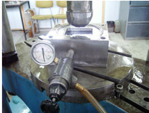
Figure 12. Photograph of the manufactured die set
