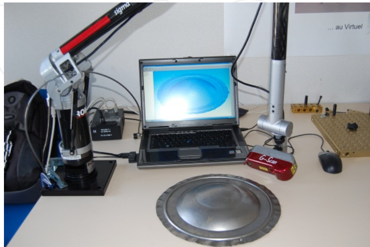
Figure 9. 3D scanner G Scan for reconstitution
