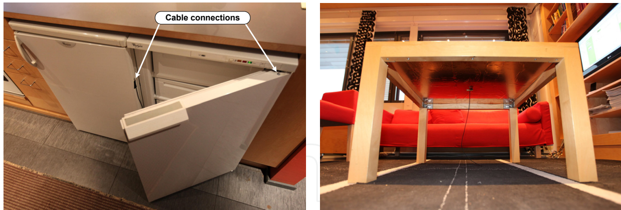
Figure 6. Both the transmitters and the receivers can be hidden in household items in order to recognize user touch and proximity to them. On the left-hand side, the metal front surfaces of the refrigerator (left appliance) and freezer (right appliance) were used as transmitting electrodes to detect when these appliances were used in the TUT Smart Home . On the right-hand side, a copper foil receiver is attached under the tabletop of the sofa table. With this receiver, the measured data was used both to detect contact with the table surface and to position the user on the floor in the vicinity of the table. The connecting cable for the receiver electrode, going under the floor through the carpet, is also visible. [51]
