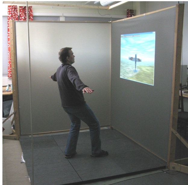
Figure 8. The electric field ranging method allows even slight body movements in the tracking space to be detected. By measuring the user distance from the vertical wires placed in each corner of the tracking space, the user position can be calculated and used in addition to indoor positioning, for example, to control a flight simulator game. [49]
