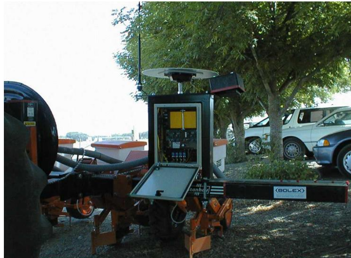
Figure 13. A RTK GPS based seed monitoring system retrofitted onto a 4-row, Salvo 650 vacuum planter
