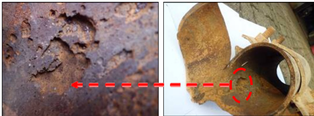
Figure 8. Wall thinning and pits at 5 – 7 o'clock position of upstream part.
