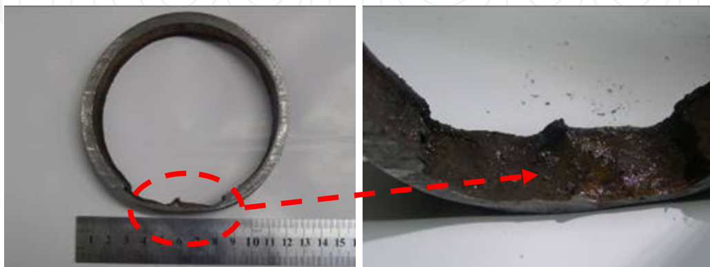
Figure 9. Uniform attack at the burst area from 5-7 o'clock position.
