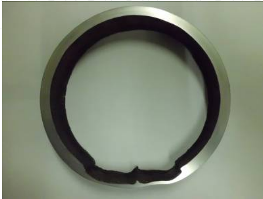
Figure 10. Results of macroetching showing the absence of ERW.
