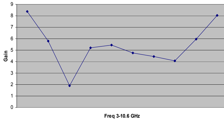
Figure 7. Antenna gain with w = 4.54\text{m} , s = 4\text{mm} and r = 40\text{mm}
