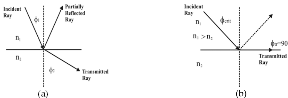
Figure 12. Snell’s law, (a) showing transmitted ray, (b) showing total reflection when critical angle is achieved.
