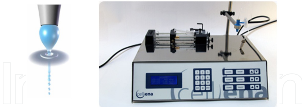
Figure 8. Flow-Focusing technology to make droplets and Cellena® equipment from Ingeniatics Tecnologías.
