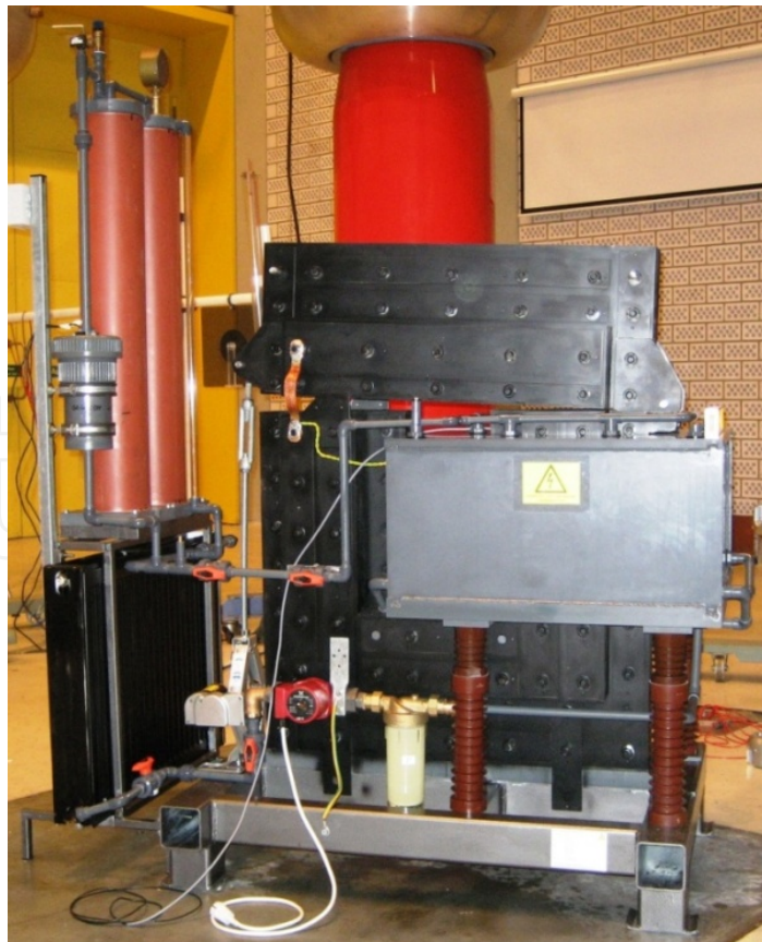
Figure 9. The resonant coil - a key ICAAS component
