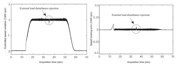
**Figure 18.** Experimental results of PSO-tuned PID-type FC implementation: fuzzy controller robustness under external load disturbance.
