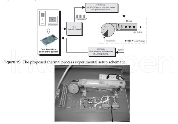
Figure 20. Developed experimental benchmark of the PT-326 Process Trainer.
