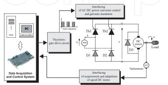
Figure 14. The proposed experimental setup schematic.
