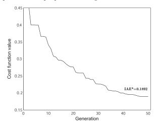
Figure 9. Convergence properties of the standard GAO algorithm: IAE criterion case.
