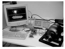
**Figure 15.** The developed experimental DC drive benchmark.
