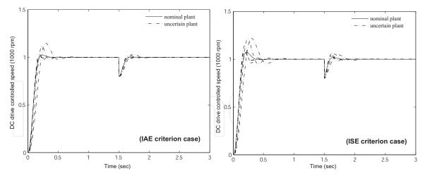
**Figure 12.** Stability robustness of the PSO-tuned PID-type fuzzy controlled system under model parameters uncertainties and external disturbances.
