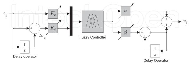
Figure 1. The proposed discrete-time PID-type FC structure.
