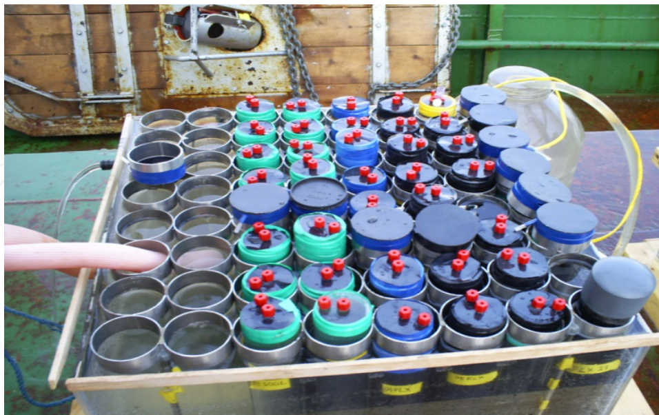
Figure 2. The incubation of core liners in the constant temperature tank on the vessel.
