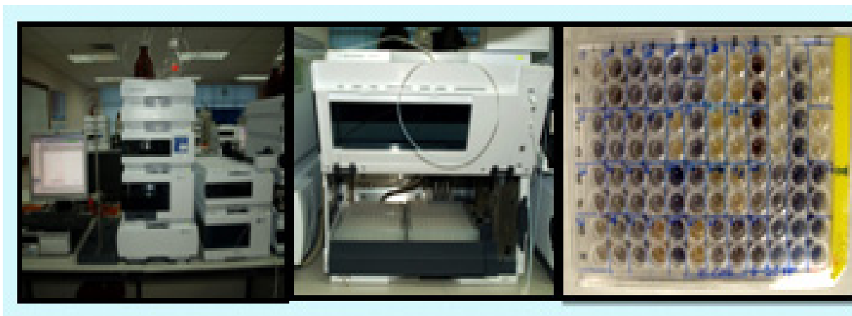
Figure 3. HPLC with DAD and ELCD detectors with fraction collector and microtitre plate.
