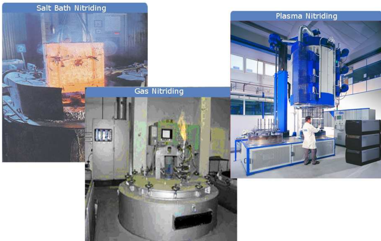
Figure 3. Commercial technologies of liquid salt bath, gas and plasma nitriding (with permission from Rubig GmbH)
