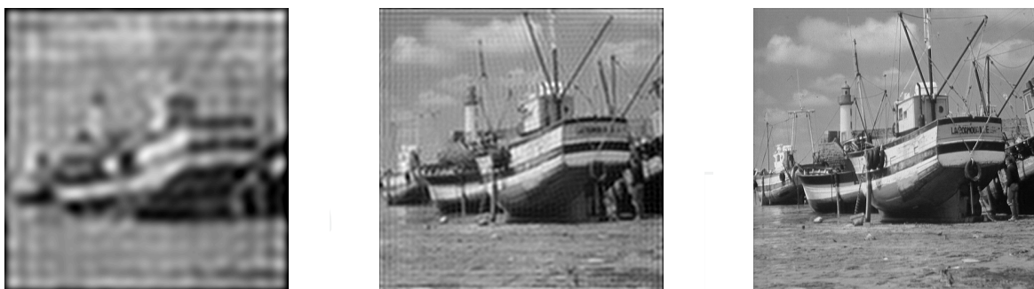
Figure 6. Fourier based moment reconstructed images for (a) k = l = 30 (b) k = l = 100 and (c) k = l = 450 .
