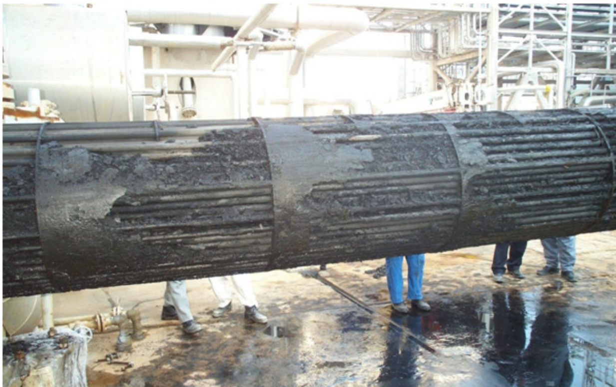
Figure 1. Fouling of heat exchangers.
