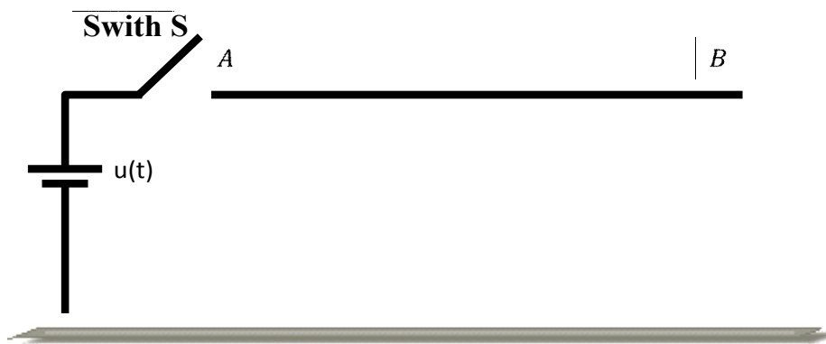
Figure 11. Single phase line representation with opened terminal.
