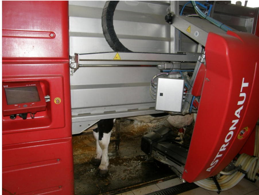
Figure 19. Computer install into AMS allowed getting the data during lactation (photo A. Váchová)
