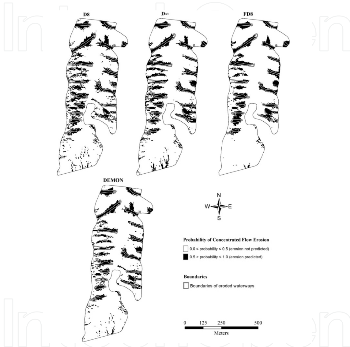
Figure 8. Discretized erosion probability maps for the logistic regression analysis of the RTK dataset comparing the D8, D_{\infty} , FD8, and DEMON flow direction algorithm.
