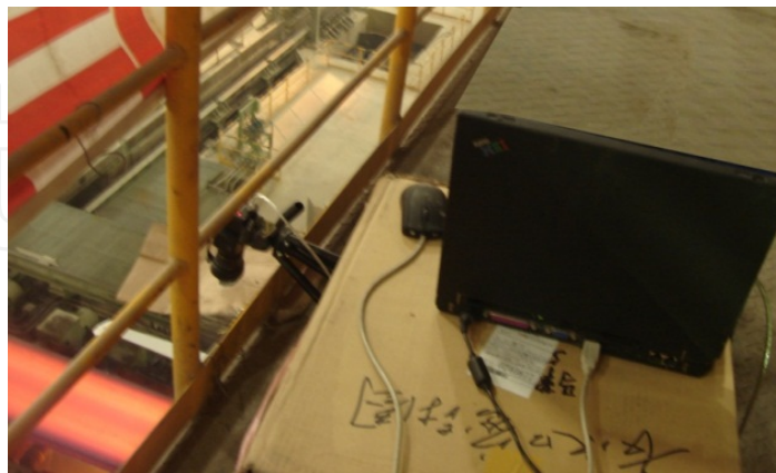
Figure 1. Online width measurement system for hot slabs. (FU JianXun et al. 2011(b))
