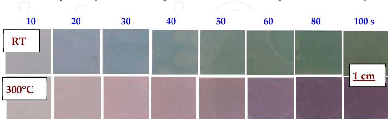
Figure 7. Images of the glass samples with gold structures sputtered for increasing times. The as-sputtered (RT) and annealed samples (300°C) are shown for comparison [16].
