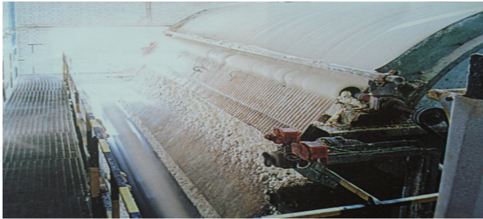
Figure 9. Pulp Screening & Cleaning in paper factory
