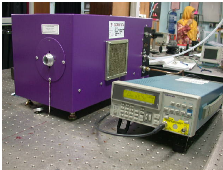
Fig. 3. An excimer laser connected to a function generator for external triggering.
