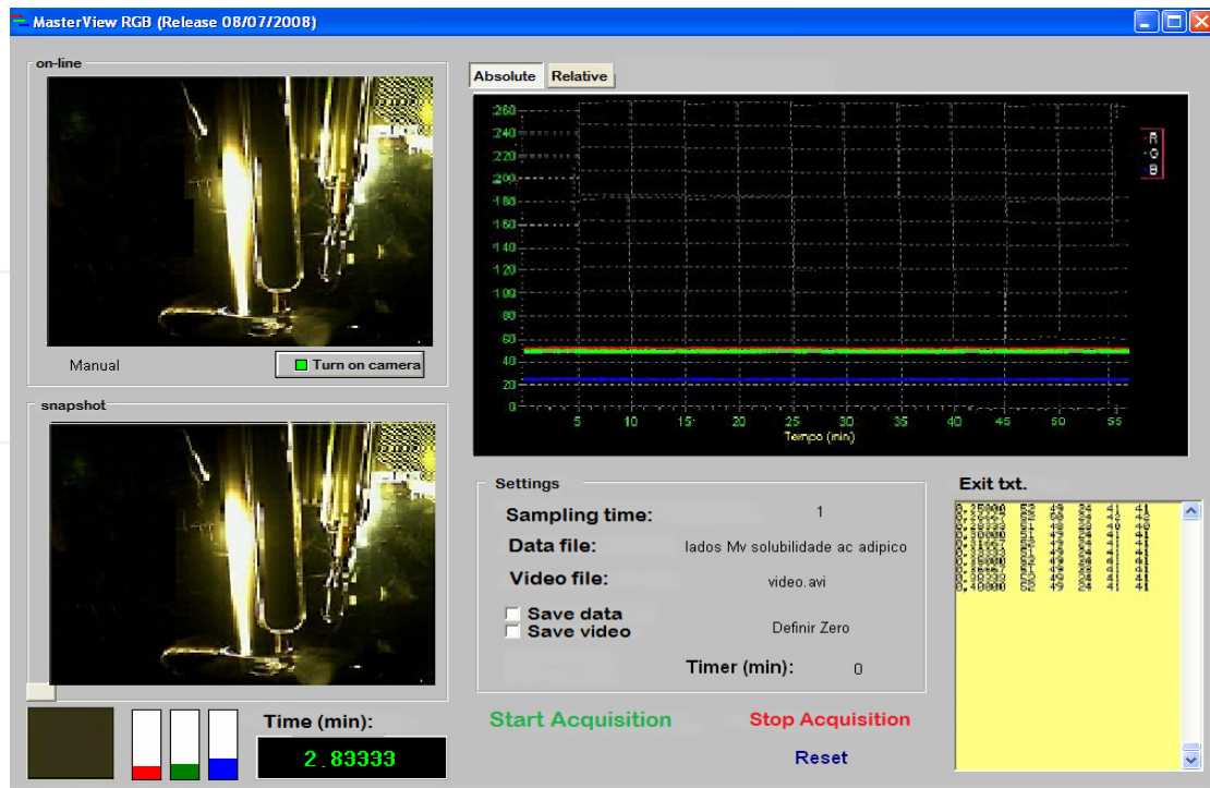
Fig. 8. Monitoring of the onset of the crystallization of adipic acid using the image analysis method (saturated solution).
