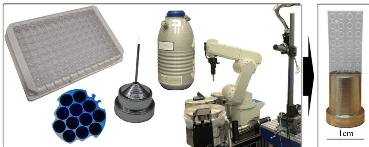
Figure 1. The X-CHIP was designed and developed as a miniaturized and integrated alternative to conventional methods of crystallization and data collection.
