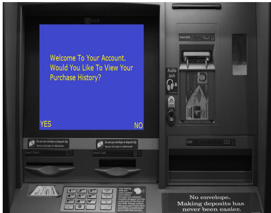
Figure 19. Adaptive Interface 5 autonomously querying the customer about viewing her purchase history, at login
