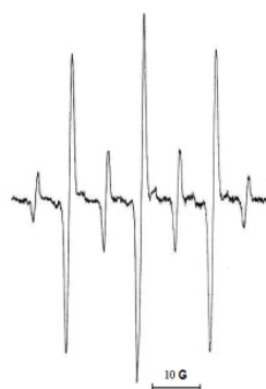
Figure 7. ESR spectra of DTBN and MNP adduct with benzyl radical observed for MNP – BC – benzene system.
