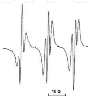
Figure 9. ESR spectra of DTBN and MNP adduct with polystyrene radical observed for MNP – PSC – benzene system
