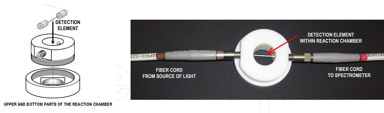
Figure 13. Schematic (a) and manufactured (b) the evanescent wave cuvette of a new design for polymerization on a side surface of the fiber core and recording the hydrogel swelling/de-swelling kinetics. The status of the hydrogel on fiber core can be controlled microscopically in the course of polymerization and swelling/de-swelling. Detection element is a removable part allowing for characterization by the other methods (e.g. atomic force microscopy).
