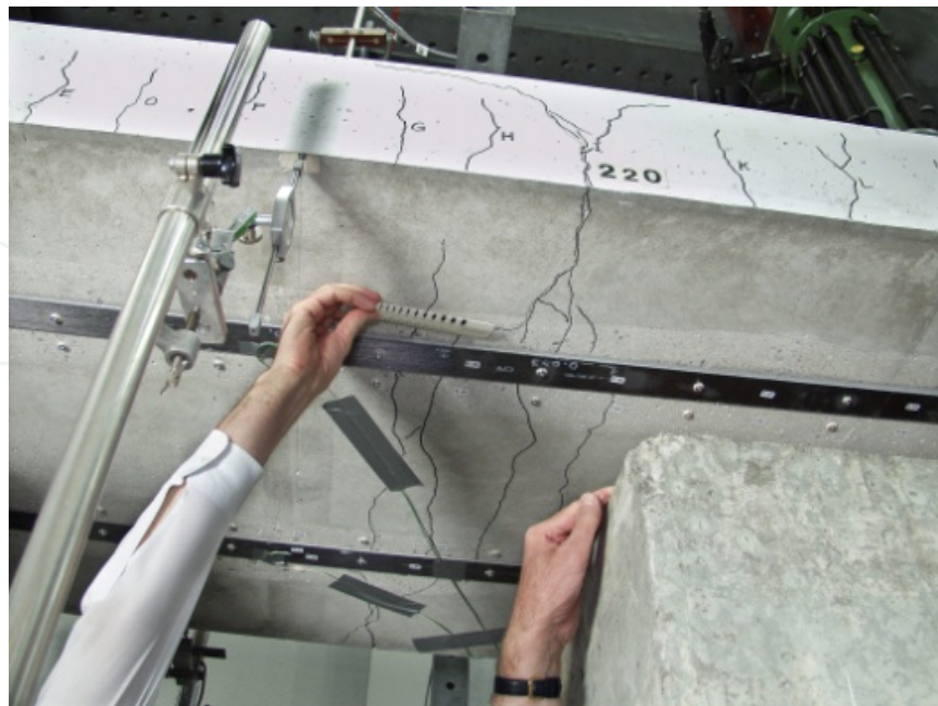
Figure 22. 2,2mm width crack at mid-span of beam VFC_PC_01 after post-strengthening failure.
