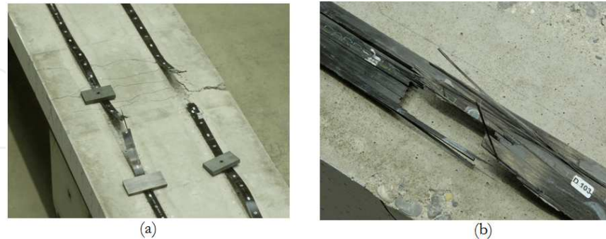
Figure 15. Failure of post-strengthening strips: (a) Next to a flexural crack; (b) Distant from flexural cracks.
