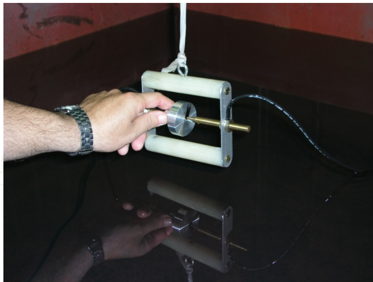
Figure 4. Device to produce partial discharges in the tank.
