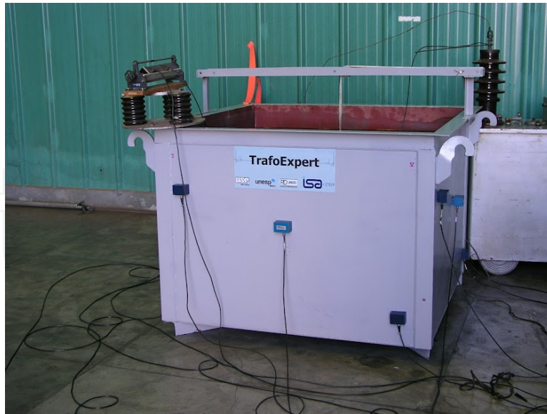
Figure 3. Acoustic emission sensor fixed to the outside of the tank.
