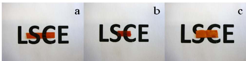
Figure 10. Qualitative evaluation of the macroscopic orientation of the different directors of the elastomeric sample by means of their optical transparency: monodomain (a), partial monodomain (b) and polydomain (c).
