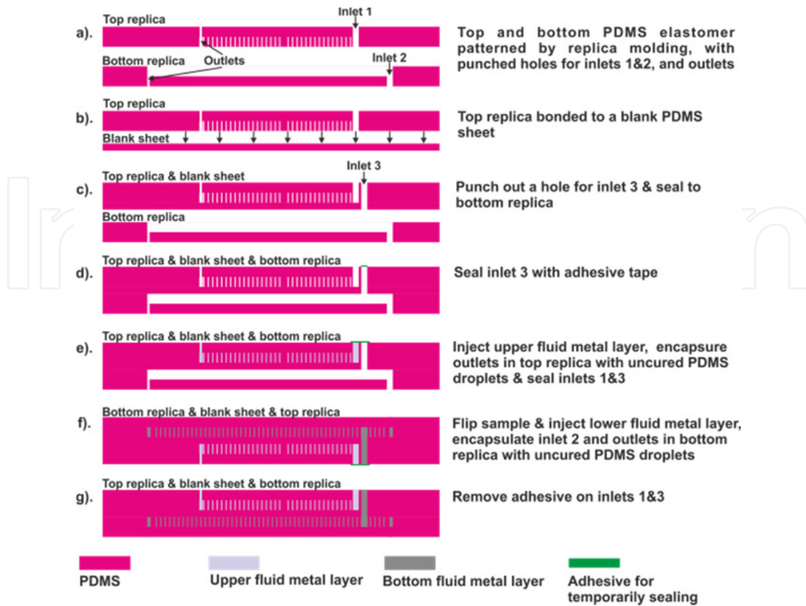
Figure 19. Fabrication process of a multi-layer microfluidics based stretchable elastomeric passive electronic device.
