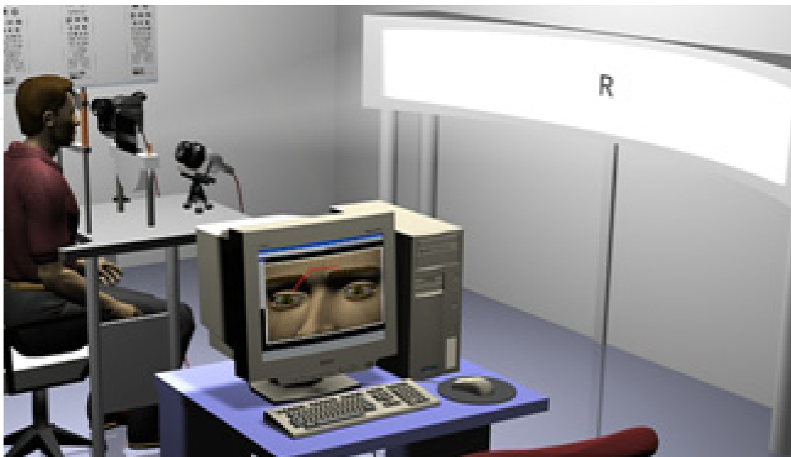
Figure 12. Video-Oculography used in DVA. It describes the subject position, Video camera matched to a PC to record the video, optotype and screen of projection.
