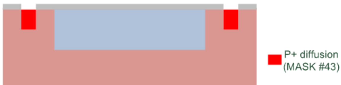
Figure 14. Guard ring get with P+ diffusion.
