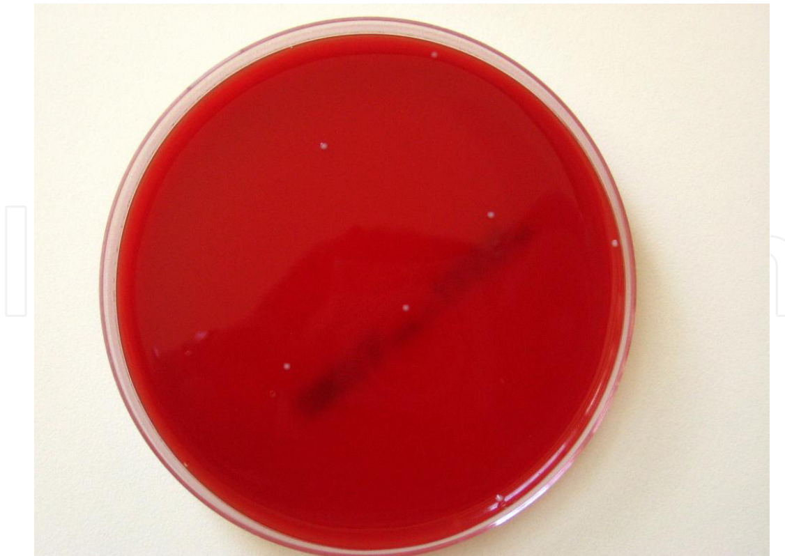
Fig. 7. The bacterial counting test for silver coated wool with E.Coli
