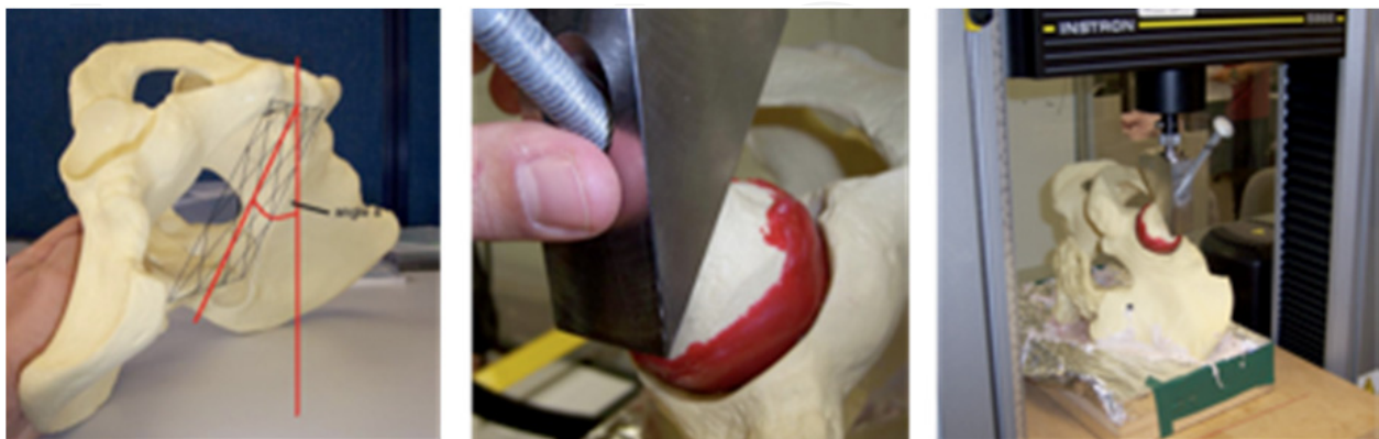
Figure 10. Photos of the experiment: The photo on the left shows the angle alpha that determined seating or standing positions; the center photo shows the close-up of the chopped femoral head attached to the holding device that goes into the crosshead of the Instron machine; the photo on the right shows the overall set-up.
