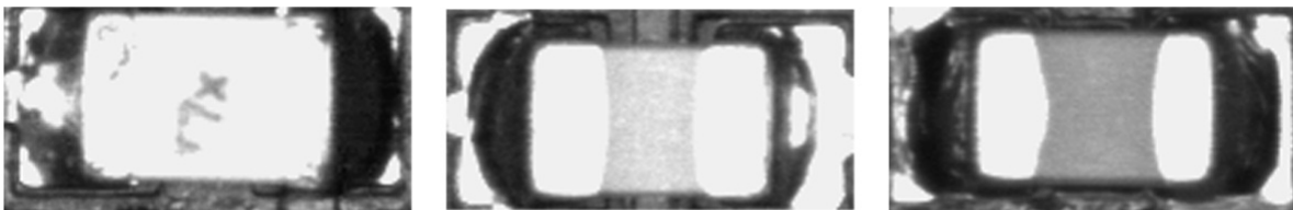
Figure 26. Differences between the appearances of similar components (capacitor C0805)
