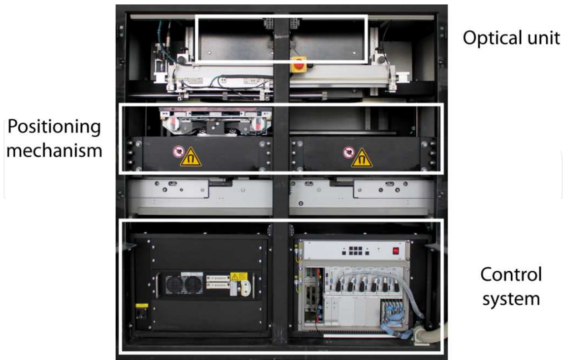
Figure 1. The three main part of an AOI system
