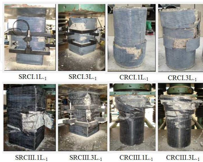
Figure 11. Typical failure modes for the tested specimens
