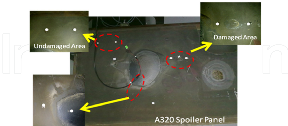
Figure 1. Locations of the structural conditions and PZT sensor placements
