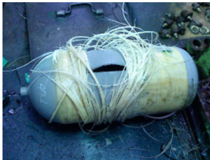
Figure 4. Composite vessel after burst test
