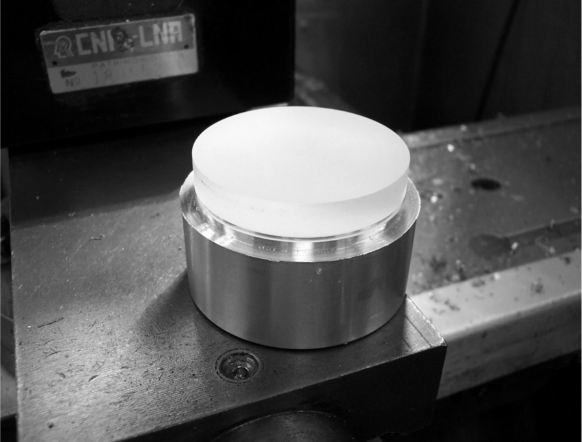
Figure 4. Plate of EPO-TEK 301-2 solidified and machined
