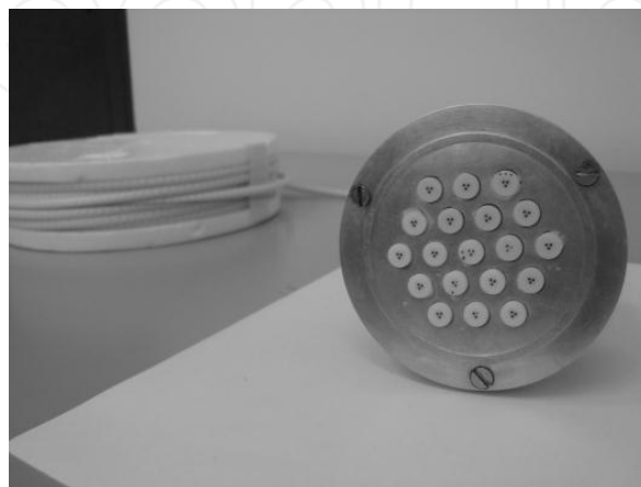
Figure 10. Inserts with optical fibres to be used in a fibres collector plate. Each insert can have several fibres.
