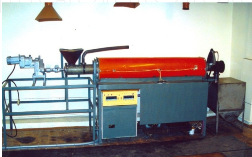
Figure 1. Pilot setup for flame carbonization of diverse raw plant materials.
