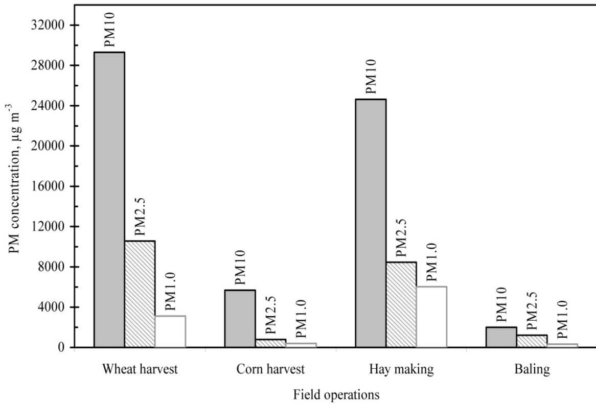
Figure 5. Particulate matter exposure in agricultural operations – predominantly organic PM sources (Arslan et al., 2010)
