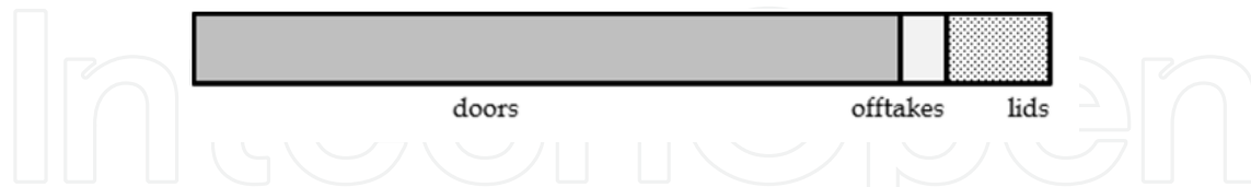
Figure 30. Spread of fugitive emissions from single leaks at the battery
