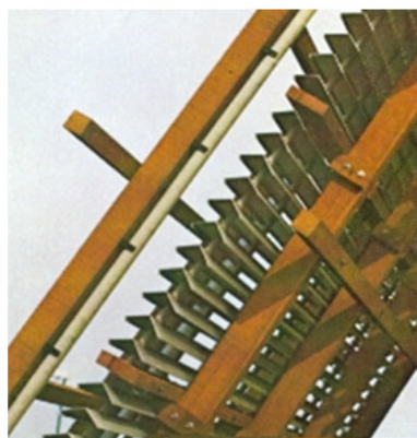
Figure 19. CSQ quench tower of the coking plant Schwelgern in contrast to the quench tower of the coking plant Huckingen (top side); bottom side: baffles (Nathaus, n.d.) for dust emission control before installation in a quench tower
