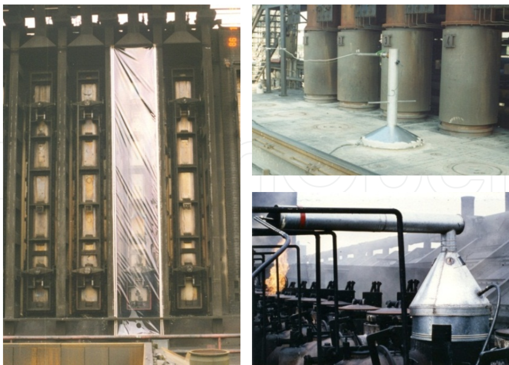
Figure 26. Equipment for measurements of fugitive emissions at doors (left side), lids (right side, top) and offtakes (right side, bottom)
