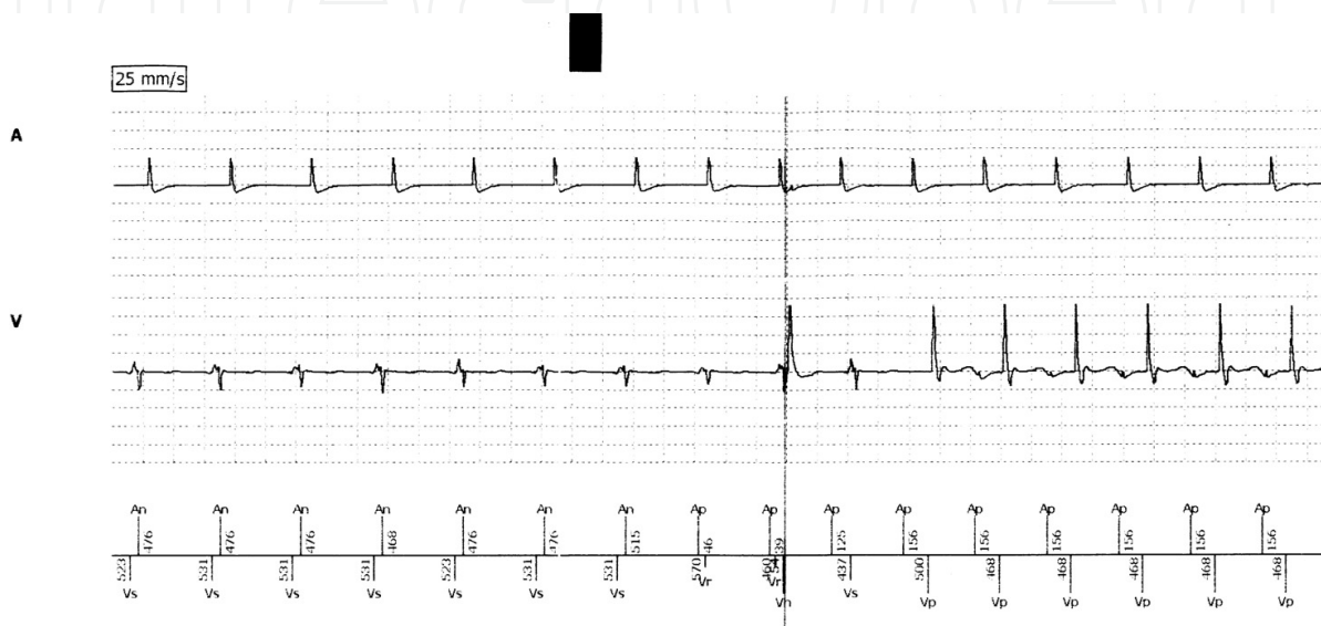
Figure 19. AAISafeR2™, Reply™ DR: With AAISafeR mode the occurrence of 2 consecutive ventricular events within the committed interval (Vr) results in mode switch to DDD. Once in DDD mode a safety stimulus is delivered here (Vn).
