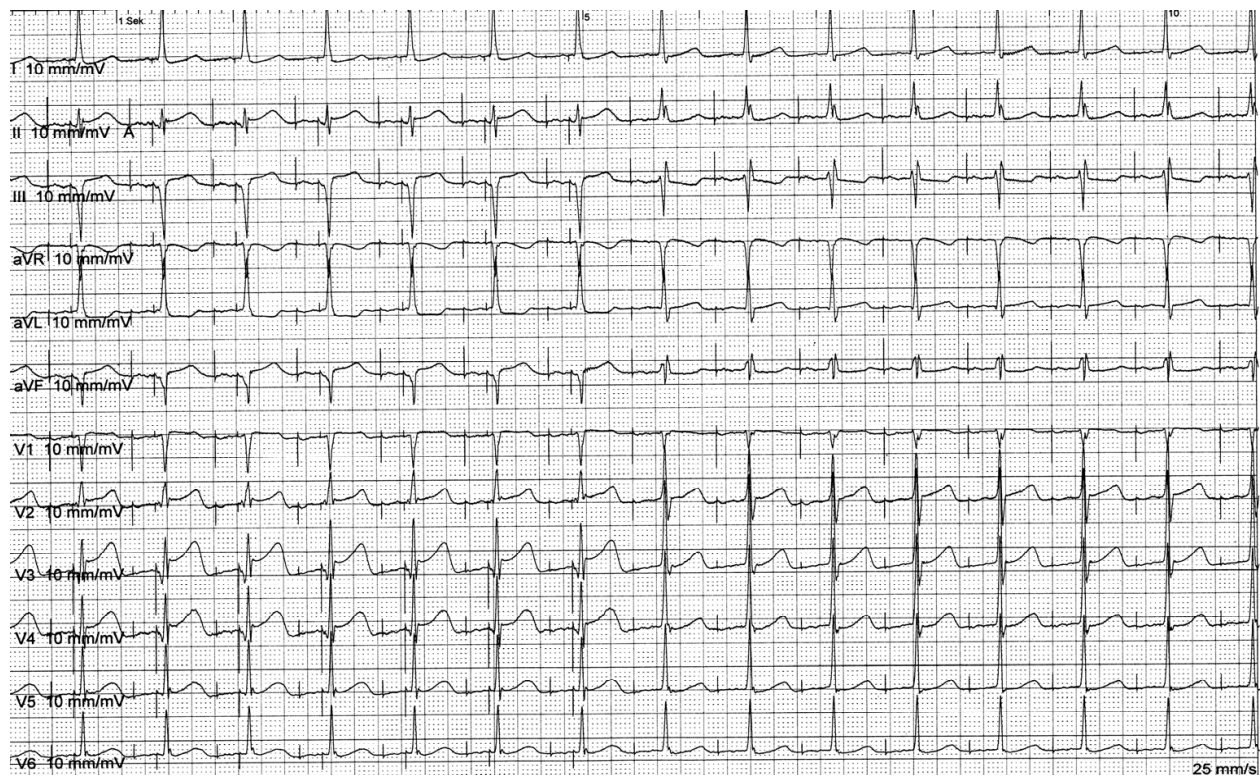
Figure 18. AAI-SafeR2™, Symphony™ DR: Successful mode switch from AV sequential DDD pacing with ventricular fusion to AAI mode resulting in intrinsic AV conduction (APace/VSense).
